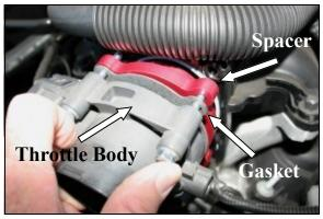
3. Install the Poweraid Spacer and the fiber gasket between the intake manifold, and the throttle body, as shown. Tighten all 4 throttle body bolts evenly, to the manufacturer's specifications. **Do Not Over Tighten The Bolts!**
