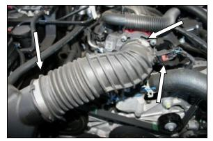
4. Reinstall the factory intake tube, and tighten the 2 hose clamps. Reconnect the wiring harness to the intake tube temperature sensor. Make sure you push down the red tab, and lock the harness. **Re-connect the negative battery cable!**
