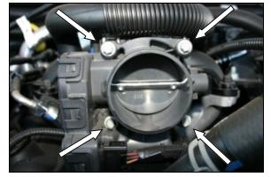
2. Using a 6 point 5/16" socket, remove the 4 bolts that hold the throttle body to the intake manifold.
