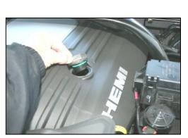
5. Remove, and set aside the oil filler cap.
