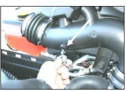
7. A.) Loosen the hose clamp on the throttle
