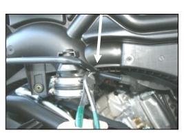
**8.** Carefully pull the resonator towards you and rotate the bottom up to gain access to the tie wrap holding the breather hose to the rubber coupler. Cut the tie wrap and discard.
