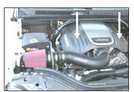
**20.** Re-align the engine cover with the grommets on the engine, and push down firmly to re-seat the cover.
