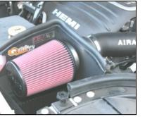
**19.** Install the Airaid Premium Filter (#1) on the Quick Fit assembly as shown, and tighten the hose clamp.
