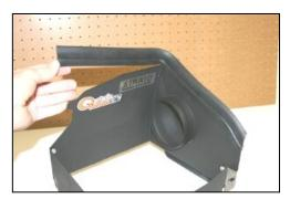
**12.** Install the weather strip (#7) on the top of the Quick Fit assembly. (Hint: start at one end, and go towards the other end, don't start in the middle.)
