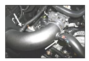
17. Very Carefully reinstall the temperature sensor removed in step #1, into the grommet in the Airaid Intake Tube. Reconnect the factory breather hose to the nipple on the intake tube.
