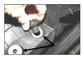
**9.** Install the 2 well nuts (#18) into the holes in the plastic air cleaner mount where you removed the grommets in step #6.
