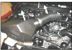
**4.** Remove the factory intake tube, and lid from the vehicle as an assembly.
