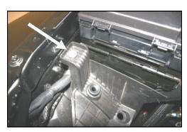
**7.** With a 10mm socket, remove and save the bolt from the factory plastic air cleaner mount. It will be re-installed in step #12.
