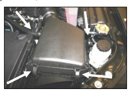
**3.** Unlatch the 4 metal clips that hold the factory air cleaner lid to the base. Next disconnect the breather hose that attaches to the rear of the air cleaner lid.
