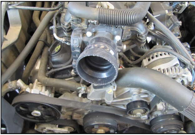
10. Slip the Hump Hose Coupler (#5) onto throttle body WITH OUT the clamps at this time.
