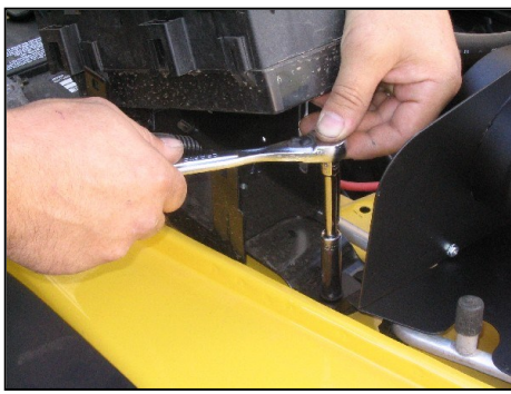
13. Align the mounting holes in the Airaid Cool Air Dam with the factory holes in the inner fender. Using the original bolts from step 7, mount the Airaid Cool Air Dam to the inner fender.
