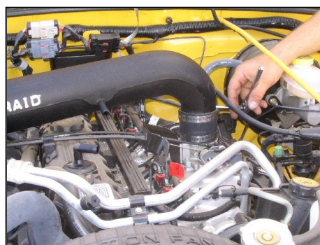
22. Install Airaid intake tube by connecting both ends into the urethane hump hose and reducer.
