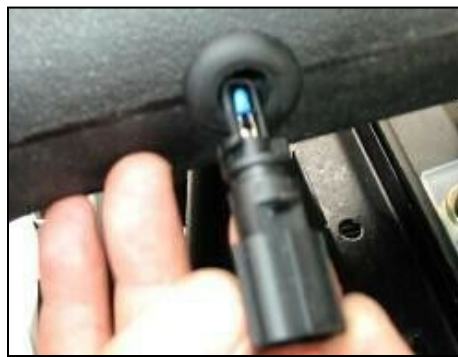
18. For 2005-06 Vehicles: Install the supplied rubber grommet with the hole. Next, install the factory air temp sensor retained from step 3 into the grommet.
