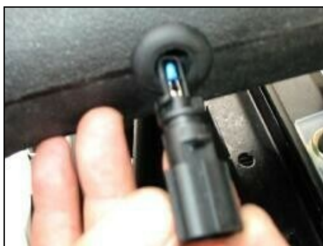
25. For 2005-06 Vehicles: Re-connect the air temp sensor on the backside of intake tube.
