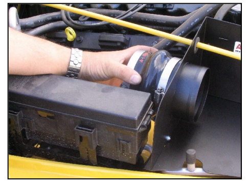
20. Install the urethane hump hose and two #72 hose clamps on end of the Airaid Cool Air Dam. Leave hose clamps loose until final assembly.
