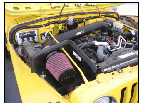
28. Install the weather strip on the edge of the Cool Air Dam assembly as shown above. Reconnect negative battery cable. Double-check your work to be certain that all nuts, bolts, and clamps are securely fastened.
