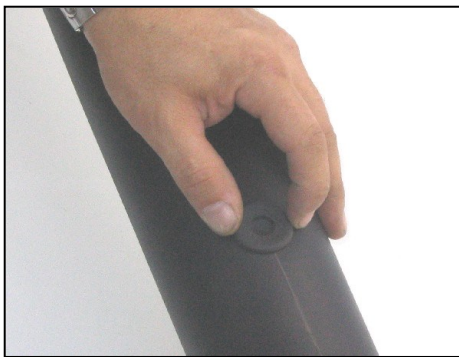
17. For 1997-2004 Vehicles Only: Install the supplied rubber grommet with out the hole into the Airaid intake tube.
