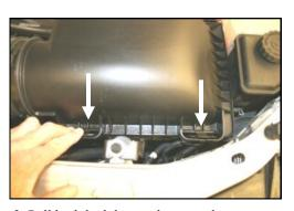
**3.** Pull both lockdown tabs towards you on the factory airbox lid to remove the lid from the base.
