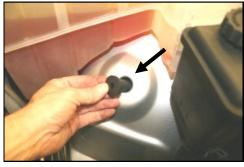
**9.** Slip the well nut (#22) into the hole in the inner fender.
