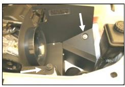
10. Install the assembled Cool Air Dam into the vehicle. Re-install the factory bolt removed in step #6 thru the CAD and into the radiator support. Next install the 3/8-16 x1 1/4" button head bolt (#10) and 3/8" flat washer (#11) thru the CAD and into the well nut. Tighten both bolts.
