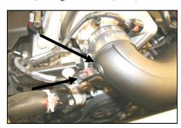
**15.** Install the grommet (#21) into the hole in the Airaid Intake Tube, and then gently push the temperature sensor (removed in step #4) thru the grommet until completely seated.
