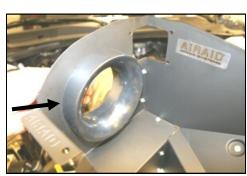
**8.** Next install the filter adapter (#6) using three  $\frac{1}{4}$  - 20 button head bolts (#12), and  $\frac{1}{4}$ " flat washers (#13).
