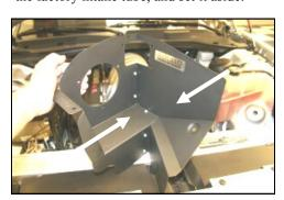
**7.** Assemble the Airaid Cool Air Dam (CAD) panels (#2, #3) using five 6-32 x 5/16" screws (#16), #6 flat washers (#17), and 6-32 keps nuts (#18).
