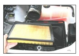
**4.** Remove the factory air filter from the bottom of the airbox.
