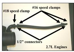
9. 2.7L Engines: Install the two 1/2" connectors (#12), into each end of the supplied breather hose (#4). Connect the breather hose to the rubber elbow on the Quick Fit Panel using one #18 speed clamp (#10), and one #16 speed clamp (#11). Install one #16 speed clamp on the opposite end of the hose as shown.
