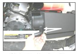
6. Slide the 1/2" rubber elbow (#8) onto the breather fitting on the side of the Quick Fit panels. Install 2 #18speed clamps (#9), one over each end of the elbow, (Do not tighten the clamps at this time.)
