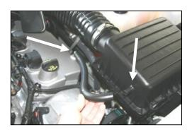
1. <u>Disconnect the negative battery cable</u>. Remove the breather hose from the factory air box lid and valve cover.
