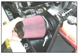
11. Slide the Airaid Premium Filter (#1) onto the Quick Fit panel tube, and tighten the hose clamp. Install the factory intake tube onto the opposite end of the Quick Fit panel tube, and tighten the hose clamp. Tighten the speed clamps on the breather hose, and the 1/2" rubber elbow.
