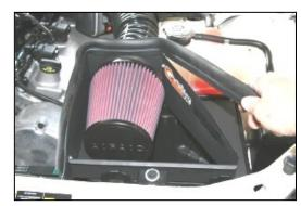
**12.** Install the weather strip (#4) on the top of the Quick Fit panels. (Hint: Start at one end and work all the way to the other end).
