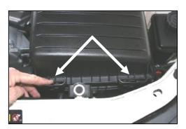
**3.** Remove the airbox lid by pulling the tabs towards the front of the car. Then, lift the lid up and slide it forward, and remove it from the bottom of the airbox.
