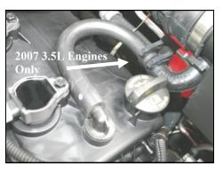
**8. For 2007 3.5L Engines**, (shown above), slide one end of the 1/2"x 1/2" connector (#10) into the rubber elbow. Slide the other end into the factory breather hose. Install one speed clamp (#9) over the factory breather hose and 1/2" connector as shown.
