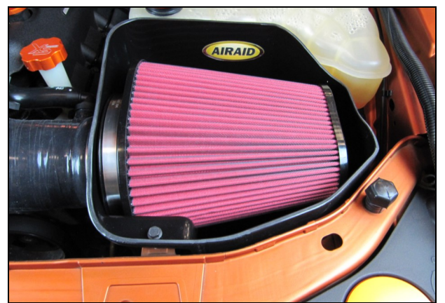
12. Install the Airaid Premium Filter onto the Filter Adapter.
