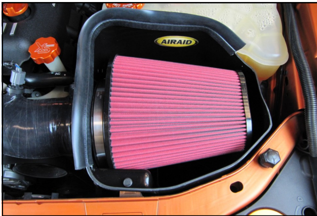
13. Install the Weatherstrip onto the top edge of the Air Box with the contour rolling away from the Filter. Reconnect the negative terminal on the battery.
