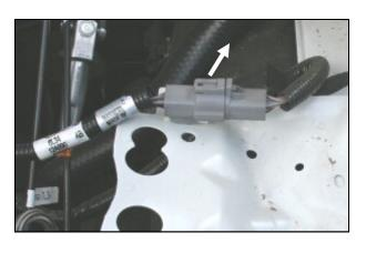
**8. 4.2L Engine Only**: Using a flat blade screwdriver, carefully pry the **MAF** sensor wiring harness connector from the holes in the airbox mounting plate (*do not disconnect it*). Move the harness towards the firewall to allow room for the **CAD** to mount.
