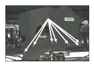
**4.** Assemble the Airaid Cool Air Dam (CAD) panels (#2, #3) using seven 6-32 x 5/16" screws (#6), #6 flat washers (#7), and 6-32 keps nuts (#8).
