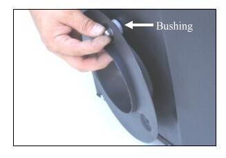
**5.** Insert three  $\frac{1}{4}$ -20 x  $\frac{7}{8}$ " bolts (#9), and  $\frac{1}{4}$ " flat washers (#10) through the **CAD**. Place one bushing (#11) at each hole between the **CAD** and the filter adapter (#4). Next, secure the assembly using three  $\frac{1}{4}$ " flat washers (#10), and  $\frac{1}{4}$ -20 nuts (#12).
