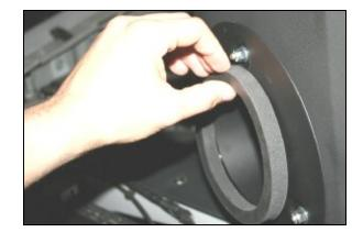
**6.** Install the supplied gasket (#13) onto the filter adapter
