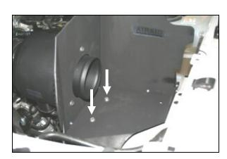
12. Insert two  $\frac{1}{4}$ -20 x 7/8" bolts (#9) and  $\frac{1}{4}$ " flat washers (#10) through the holes in the CAD and thru the grommets. On the underside of the factory airbox mounting plate, align the long/narrow bracket (#16), two  $\frac{1}{4}$ " flat washers (#10), and two  $\frac{1}{4}$ -20 nuts (#12) with the  $\frac{1}{4}$ -20 x 7/8" bolts. Tighten the assembly securely.
