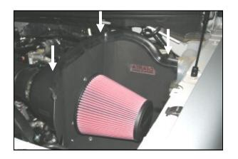
**14.** Install the weather strip (#5) onto the top edge of the **CAD** as shown. (*Hint: start at one end and work your way around to the other.*)
