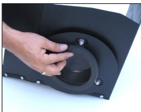
5. Install the supplied gasket on the Airaid filter adapter as shown.
