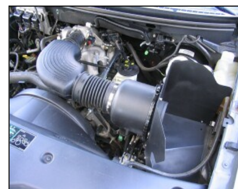
8. Install the Airaid Cool Air Dam assembly on vehicle using the factory intake tube clamp.
