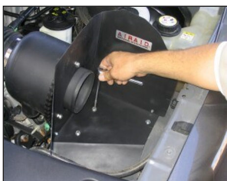
10. Finish mounting the Airaid Cool Air Dam assembly to body using the supplied 1/4" nuts, bolts, washers and long bracket as shown. Note: The long bracket must be mounted under the factory mounting plate and grommets.
