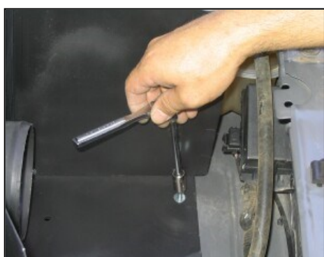
9. Mount the Airaid Cool Air Dam assembly to the vehicle using the supplied metric bolt and washer and the factory bolt hole as shown above.
