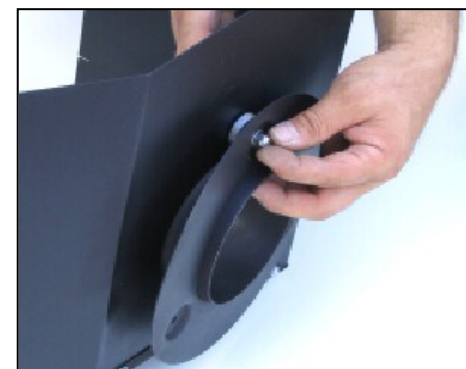
4. Assemble the Airaid Filter Adapter plate using the supplied 1/4 inch bolts, washers, spacers and nuts provided as shown above.
