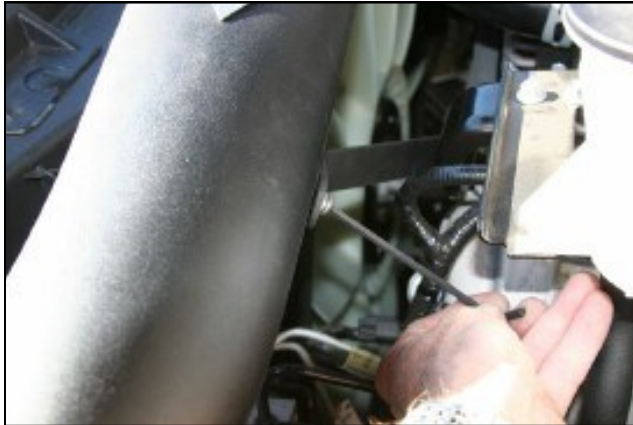
14. Install a 1/4-20 Allen bolt and flat washer thru the bracket at the back of the tube, and tighten. Tighten the nut at the bottom of the bracket. Tighten the hose clamps on the hump hose.
