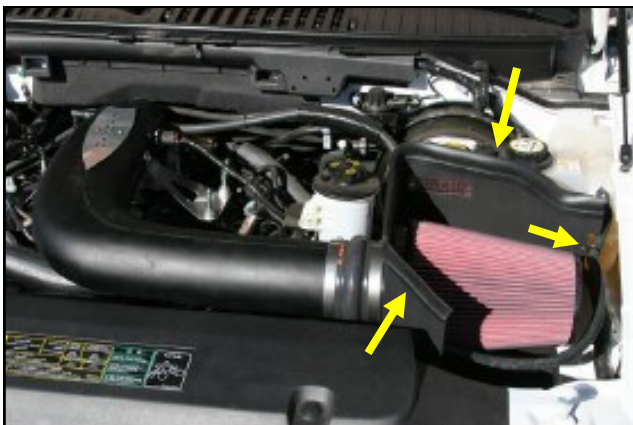
17. Install the weather strip on top of the cool air dam. (Hint: Start at one end and work towards the other for an easier fit.) Spread the two hose mounts over the radiator overflow hose, and insert one in each hole at the ends of the cool air dam.
