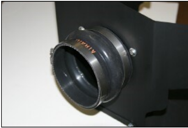
11. Install the urethane hump hose and two #72 hose clamps. (Leave loose until final adjustments are made.)
