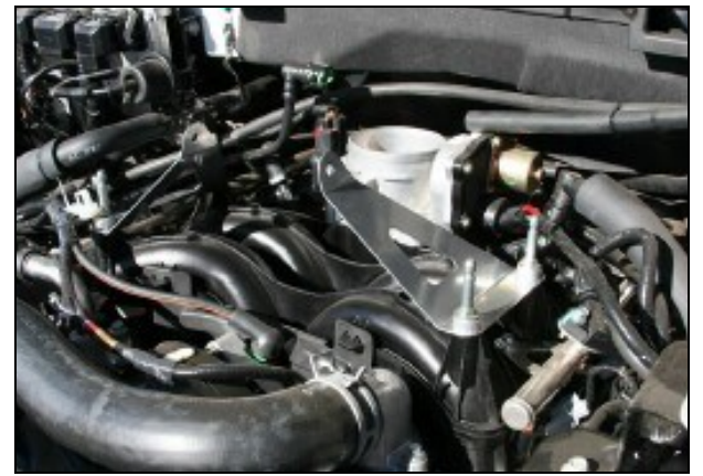
12. Install the two Airaid intake tube brackets on the top of the intake manifold, using the four aluminum spacers on top of the bracket and the four tower bolts. (Leave loose until final adjustments are made.)
