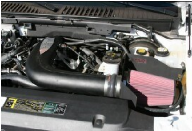
16. Install the Airaid Premium Filter inside the cold air dam.
