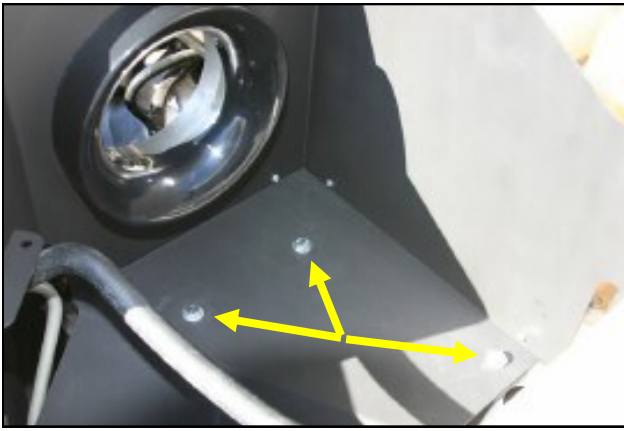
10. Mount the Airaid Cool Air Dam assembly to the vehicle using the supplied metric bolts and washers. The bolt on the right goes into the factory threaded hole. The two bolts on the left go thru the CAD, the grommets, and then the supplied bracket, with the nuts on the bottom. (Note: The mounting bracket must be on the bottom of the grommets.)
