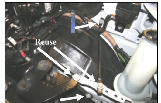
6. Using a 1/2" socket, ratchet and extension, remove the 2 bolts that hold the support rod, and 2 bolts that hold the air cleaner base support. Remove the support rod and base support and set them aside. The 2 bolts that hold the air cleaner base support will be reused in step #11.
