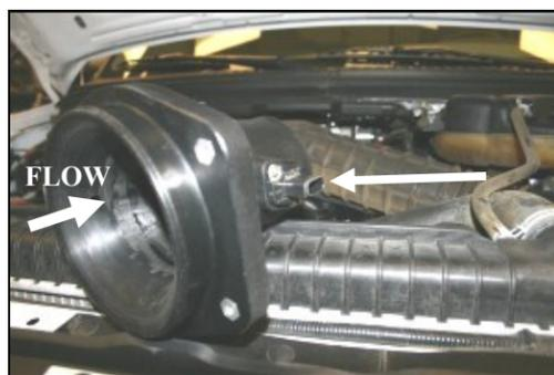
5. Install the factory mass air sensor into the Airaid MAF Adapter (#4), using the two supplied 8-32 button head screws (#9) and a 3/32" allen wrench. Note the direction of flow on the sensor, and mount as shown above. **DO NOT USE THE FACTORY SCREWS!!**
