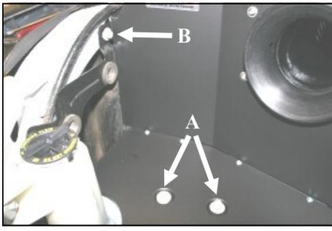
11. A.) Align the two panel holes with the air cleaner base support holes on the vehicle. B.) Align the tab on the panel with the radiator support bolt hole. The tab will mount on top of the bracket. Re-install the bolts saved from steps #6 and #7 into the two bottom holes of the Cool Air Dam, and one through the radiator support tab.
