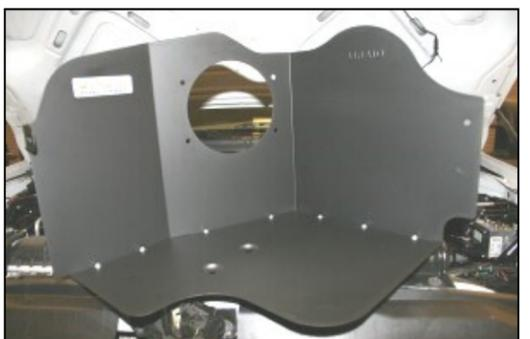
9. Assemble the two Cool Air Dam panels (#2 and #3) as shown, using seven 6-32 screws (#10), #6 washers (#11), and keps nuts (#12). Tighten securely.
