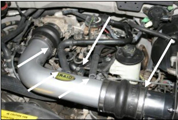
10. Reinstall the air intake tube and tighten the two hose clamps. Reconnect the two rubber hoses to the intake tube. Reconnect the air intake temperature sensor wiring harness. Reinstall the engine beauty cover using the three factory bolts from step #1.
