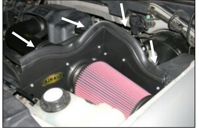
12. If your vehicle Does Not have a hood mat, install the panel extension (#4) as shown using five 6-32 Phillips head screws (#5), flat washers (#6), and kep nuts (#7). Next install the weatherstrip (#4) onto the top of the panel assembly as shown.
