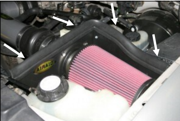
11. If you Do have a hood mat, install the Airaid Premium Filter onto the MAF bracket and tighten the filter. Next install the weatherstrip (#4) onto the top of the panel assembly as shown. If your vehicle Does Not have a hood mat, proceed to step # 12.
