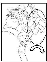
15. 4.6L engines: The idle air bypass line goes directly to the throttle body. Rotate the resonator box 90 degrees to provide clearance for the 3/4 x 12" L-hose (#7). Install the 3/4"x12" L-hose (#10) onto the Airaid Intake tube and the resonator box and secure it using the two #22 speed clamps (#23)
