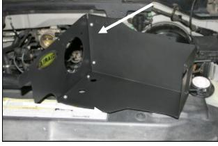
**6.** Assemble the MAF panel (#3), and bottom panel (#4) as shown using four 6-32 screws (#12), four flat washers (#13), and four Kep nuts (#14) as shown.
