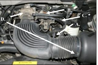
2. A) <u>Very carefully</u>, using a pulling circular motion, remove the air intake temperature sensor from the air intake tube. B) Disconnect the upper, idle air bypass hose. C) Disconnect the crankcase breather at the intake tube and the valve cover, and remove it from the vehicle. D) Loosen two hose clamps and remove the air intake tube from the vehicle.
