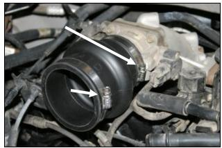
**12.** Install the small end of the reducing hump hose (#8) onto the throttlebody and tighten the #52 hose clamp (#20). Next, install the remaining #60 hose clamp (#21) on the large end of the hump hose leaving it loose for now.
