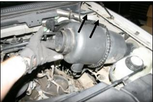
**3.** Lift straight up on the outlet side of the air filter canister to remove it from it's locating grommets. Next, pull it towards the engine to dislodge it from the inner fender well.
