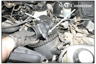
4.Unlatch the clamp on the canister to separate the two halves. Once separated, remove the factory air filter.
