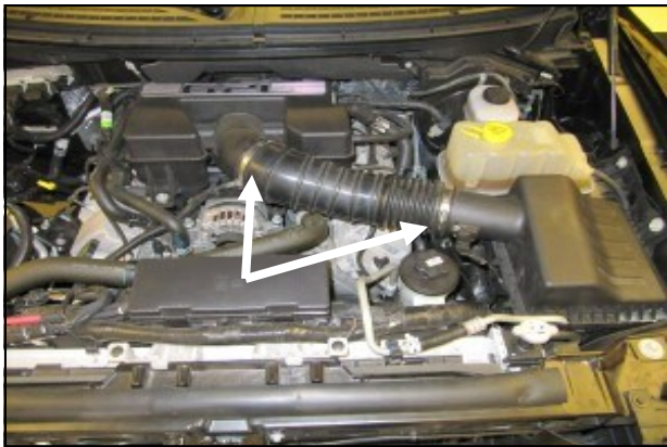
1. Disconnect the negative battery cable! Loosen the two intake clamps and remove the Factory intake tube.
