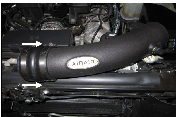
7. Install the Hump Hose (#5), and the clamps (#13) onto the Intake Tube. Slide the hump hose and clamps down the tube as far as they will go and leave the clamps loose for now.
