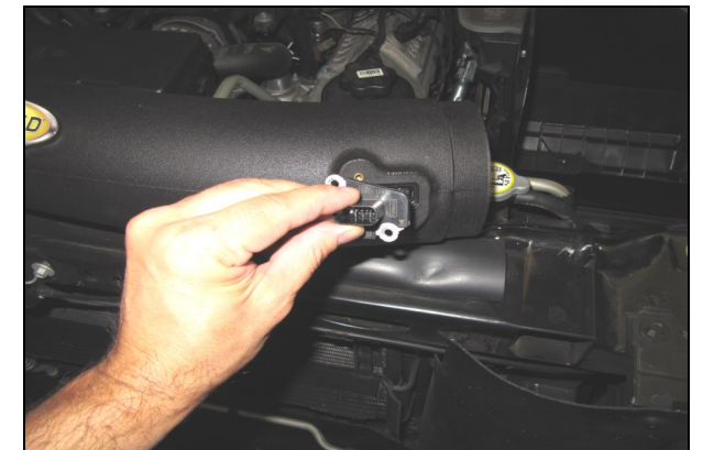
6. Transfer the MAF sensor into the Airaid Intake Tube (#2) and secure using two 8-32 x 1/2" button head screws (#10). Do Not Use The Factory Torx Head Screws
