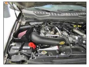
16. Double check your work! Make sure there is no foreign material in the intake path. Make sure all clamps, hoses, bolts, and screws are tight. Double check the hood clearance! Reconnect the negative battery cable!
