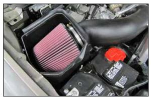
13. Install the air filter onto the intake tube and secure with the provided hose clamp.
