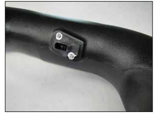
11. Remove the mass air sensor from the factory air filter housing and install it into the AIRAID® intake tube using the provided hardware and spacers. Install the AIRAID<sup>®</sup> decal onto the intake tube.
