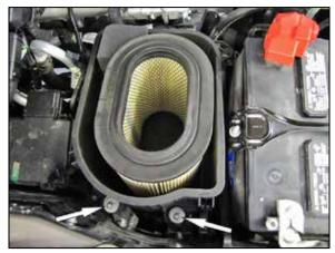
4. Remove the two bolts that secure the lower air filter housing to the mounting bracket, then pull the lower air filter housing straight up to dislodge it from the mounting grommets and remove it from the vehicle. **NOTE: AIRAID recommends that customers do not discard factory air intake.**  5. Remove the two bolts that secure the air filter housing mounting bracket to the inner fender and remove the bracket from the vehicle.
