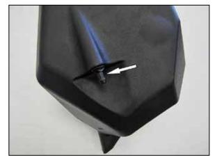
6. Install the provided air box mounting stud onto the AIRAID<sup>®</sup> housing using the provided hardware.
