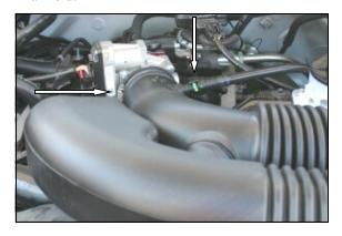
**5.** Re-install the factory intake tube onto the throttle body and tighten the hose clamp. Re-connect the breather hose to the factory intake tube. **Re-connect the negative battery cable!**
