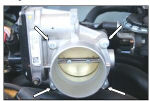
**2.** Remove the four bolts (and/or nut and stud) from the throttle body, and remove the throttle body from the intake manifold, and set it aside. Retain the wiring harness anchor from the upper left stud on the Explorer for reinstallation in step #4.
