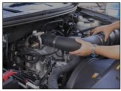
**7.** Install the Airaid Modular Intake Tube on engine.
