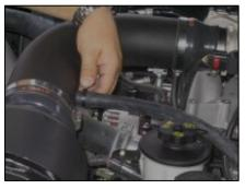
9. Install the supplied rubber hose on the Modular Intake Tube. Connect the other end of the hose to the valve cover. Secure both ends of the hose with the supplied speed clamps.
