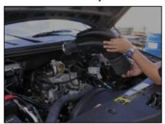
**3.** Remove the factory intake tube assembly from engine.
