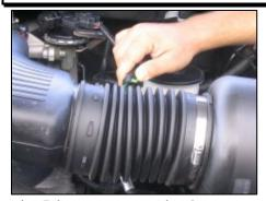
1. Disconnect negative battery cable. Disconnect valve cover breather hose from factory intake tube and valve cover.
