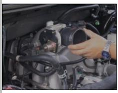
6. Install supplied silicone reducer on end of throttle body. Install #48 hose clamp on small end of the reducer and #56 hose clamp on the big end of the reducer. Leave hose clamps loose until final assembly.
