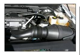
1. Disconnect negative battery cable. Disconnect intake tube from air filter housing by unsnapping the tube assembly from the housing.
