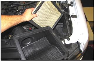
**3.** If installing the Airaid Jr. Kit, unfasten the three clips on the left side of the factory airbox, and remove the upper half of the factory airbox. Remove the factory air filter element.
