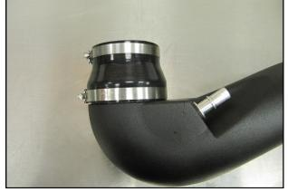
**8.** Install the Silicone Reducer (#4) and Hose clamps onto the Airaid Intake Tube. Place the #56 Clamp (#18) on the throttle body side of the Reducer, and the #64 Clamp (#9) on to the Tube side.
