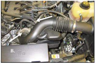
**2. A.** Disconnect the two breather lines in the factory intake tube .
