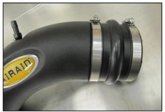
**7.** Install the hump hose (#3) and two #60 hose clamps (#9) onto the Intake Tube as shown. Leave the hose Clamps loose for now.
