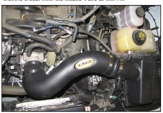
**9.** Install the Intake Tube onto the throttle body first, then into the airbox. Tighten all of the Hose Clamps.
