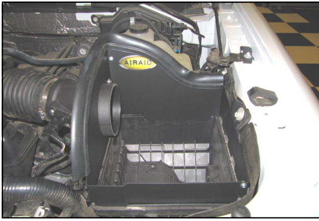
10. Install the Weather Strip (#5) to the Panel assembly as shown, with the contour rolling away from the filter area.
