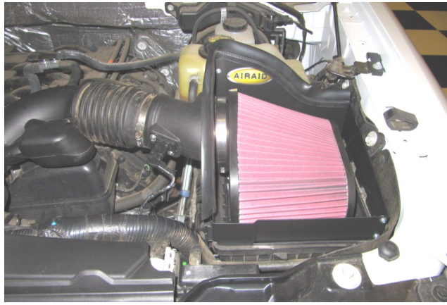
11. Install the Airaid Premium Filter (#1) on to the Air Meter Tube and tighten the clamp.
