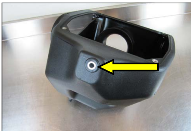
7. Insert the 5/8" Grommet and Spacer into the opposite side of the Airaid Air Box.
