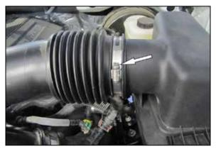
3. Loosen the hose clamp that secures the factory intake tube to the upper air filter housing.
