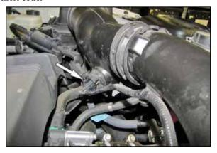
2. Disconnect the inlet air temperature sensor electrical connection.
