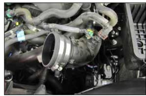
7. Install the provided coupler hose (08761) onto the driver's side turbo inlet tube and secure with the provided hose clamp.
