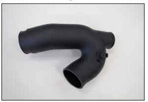
10. Using the provided grommet, install the factory inlet temperature sensor into the AIRAID intake tube as shown.
