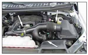
3. Loosen the three hose clamps that secure the factory intake tube and then remove the intake tube from the vehicle.
