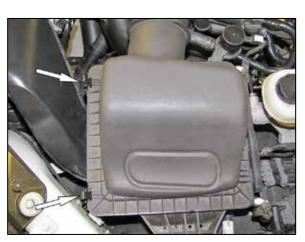
4. Release the two clips that secure the upper air filter housing and then remove the housing and factory air
