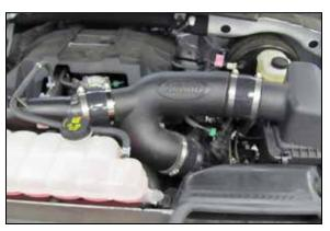
10. Install the factory upper air filter housing into the tube on the coupler and onto the lower filter housing. Secure with the factory retaining clips and hose clamp provided.
