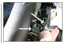
7. Install the 1/4"x 20 Allen bolt and washer thru the bracket and into the MIT. Make your final adjustments and tighten the Allen bolt, and the nut on the power steering bracket. The MIT should not make contact with the radiator support or inner fender.
