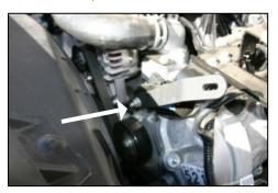
3. Remove 13mm nut on power steering reservoir bracket. Install Airaid Modular Intake Tube support bracket, replace nut, and leave slightly loose. (Nut will be tightened after final adjustments.) 4. <u>Airaid Jr. Kit PN#401-766</u> If you purchased the Airaid Jr. Kit PN#401-766, replace the factory air filter with the Airaid Premium filter PN#850-349 included with the kit.
