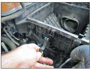
12. Remove the center airbox retaining clip.
