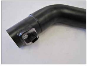
18. Install the mass air sensor into the AIRAID<sup>®</sup> intake tube and secure with the provided hardware.
