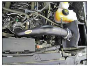
19. Install the AIRAID<sup>®</sup> intake tube assembly into the hose at the filter adapter and then into the hose on the throttle body and secure with the provided hose clamps.
