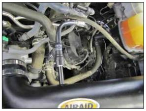
20. Connect the crankcase vent hose to the quick disconnect fitting on the AIRAID<sup>®</sup> intake tube.
