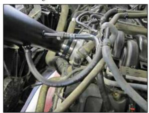
11. Install the AIRAID<sup>®</sup> air filter onto the filter adapter and secure with the provided hose clamp.
