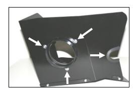
**10.** Install the air filter adapter (#2) into the **CAD** using three  $\frac{1}{4}$  - 20 x 1/2" button head bolts (#14) and  $\frac{1}{4}$ " flat washers (#15). Next, install the 4" rubber trim (#23), as shown.
