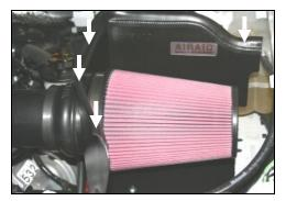
**19.** Install the Airaid Premium Filter (#1) onto the air filter adapter (#2), and tighten the clamp. Next install the weather strip (#9) onto the top of the **CAD** as shown. (*Hint: start at one end of the CAD and work towards the other end*).
