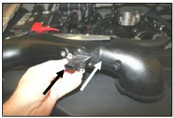
**5.** Re-install the **MAF** sensor into the Airaid Intake Tube (#5) using two 8-32 x 3/8" button head screws (#10). **Do not over tighten! Do Not Use The Factory Screws!!**
