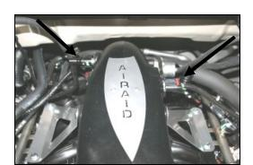
**20.** Re-connect the breather hose to the Airaid Intake Tube, and the **MAF** sensor wiring harness to the sensor. Refer to step #1.
