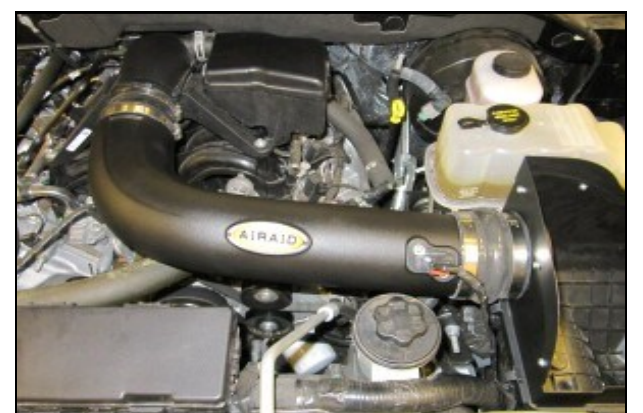
9. A.) Insert the Airaid Intake Tube into the couplers as shown. Check for alignment, and tighten all clamps. B.) Re connect the Mass Air Flow Sensor.
