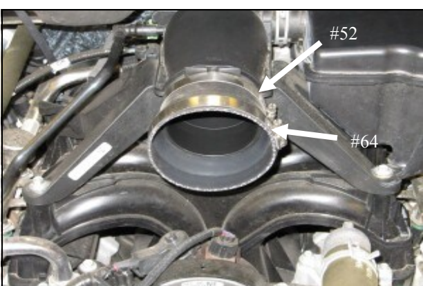
7. Install the Silicone Coupler (#6), one #64 Hose Clamp (#14), and the #52 Hose clamp (#13) onto the engine air inlet. Leave the clamps loose for now.
