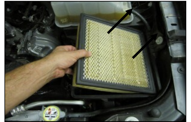
3. Remove the factory air filter from the lower half of the airbox.
