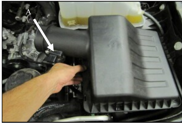
2. A.) Disconnect the Mass Air Flow (MAF) Sensor. B.) Unfasten the three airbox clips on the left side, and remove the upper half of the factory airbox.
