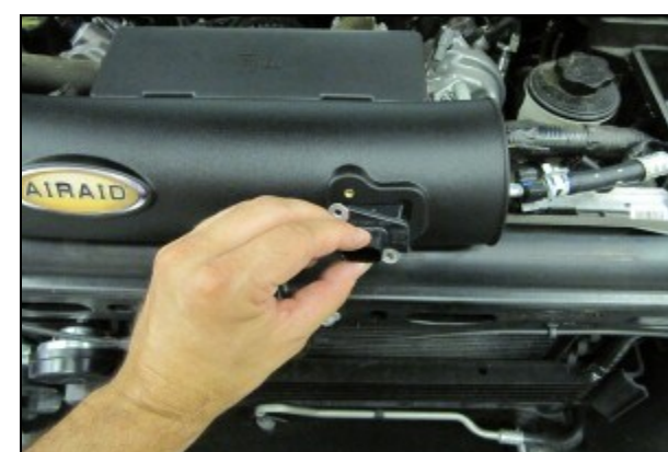
8. Transfer the MAF sensor into the Airaid Intake Tube (#2) and secure using two 8-32 x 1/2" button head screws (#11). Do Not Use The Factory Torx Head Screws!
