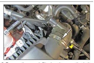
5. Remove the rear air filter housing mounting bolt and loosen the hose clamp that secures the intake hose to the housing.
