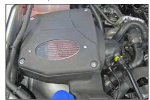
16. Install the lid onto the filter housing and secure with the provided hardware.
