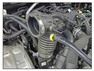
7. Loosen the hose clamp that secures the intake hose to the plenum and then remove the hose from the vehicle.
