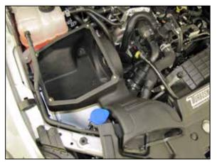
9. Install the AIRAID® air filter housing assembly and secure the air filter housing with the factory hardware and the fresh air duct with the hardware provided.
