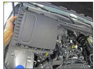
6. Remove the air filter housing from the vehicle. NOTE: AIRAID recommends that customers do not discard factory air intake.
