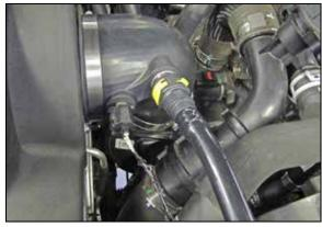
14. Reconnect the inlet air temperature sensor electrical connection and connect the crank case vent line to the quick connect fitting as shown.
