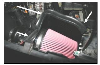
**13.** Install the supplied weather strip (#7) onto the top of the **CAD** starting at the fender and working your way towards the radiator.
