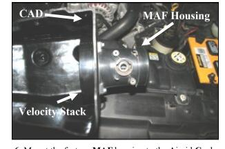
**6.** Mount the factory **MAF** housing to the Airaid Cool Air **D**am (#6) using four 6mmx25mm bolts (#8), four lock washers (#10), two MAF gaskets (#12), and one velocity stack (#3). Refer to the line drawing at the top of this page for the proper sequence of how to install the parts.
