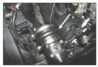
**10.** Install the hump hose (#5) onto the factory **MAF** housing using two #60 hose clamps (#15) as shown. Tighten *only* the clamp on the housing at this time.
