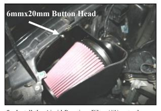
9. Install the Airaid Premium Filter (#1) onto the velocity stack inside of the CAD as shown and tighten the clamp. Next install the CAD assembly into the vehicle aligning the grommet posts into the factory grommets in the inner fender. Now secure the CAD to the inner fender well using the 6mmx20mm button head bolt (#9), and flat washer (#11).
