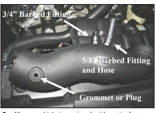
7. If your vehicle is equipped with an intake temp sensor (1999-01), install the supplied grommet (#17) into the hole in the Airaid Intake Tube (#2), On later models (2002-04), install the grommet plug (#18). Next install the two barbed fittings (#19 & #20) into the tube as shown. Now install the 5/8"x 3" hose (#16) onto the 5/8" barbed fitting.
