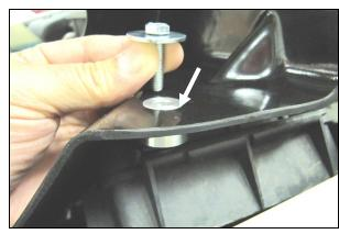
12. Slide the Aluminum Spacer (#12) underneath the CAD and into the hole as shown. Secure the CAD to the inner fender using the OEM bolt from step #1 and the supplied 1/4" Fender Washer (#10).
