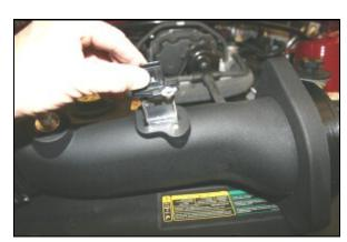
9. Install the Mass Air Flow sensor removed in step #5, into the Airaid Intake Tube using the provided 8-32 x 3/8" button head screws (#8). Make sure the arrow on the sensor is pointing towards the throttle-
