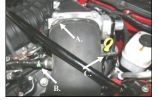
2. A.) Loosen the factory intake tube hose clamp on the throttle body. B.) Push the GREEN tab on the breather hose connector and disconnect it from the factory intake tube. C.) CAREFULLY disconnect the vacuum line from the factory intake tube.
