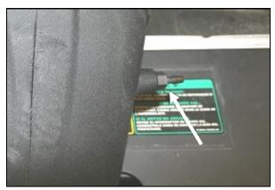
8. Install the 1/8"NPT x 3/16" barbed fitting (#13) into the small threaded hole in the side of the Airaid Intake Tube.
