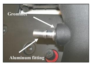
7. Install the provided grommet (#11) into the large hole in the side of the Airaid Intake Tube (#2). Next, carefully install the supplied aluminum fitting (#14) into the grommet as shown.
