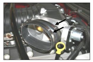
10. Install the oval hump hose (#4) onto the throttle body with two provided #80 hose clamps (#9). Leave the clamps lose for now.
