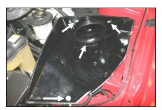
13. Install the Cool Air Dam into the vehicle aligning the grommet posts on the bottom of the CAD into the factory grommets in the fender well. Now install three 1/4" button head bolts (#6) and flat washers (#7) thru the CAD and into the Airaid Intake Tube. Next reinstall the second factory bolt from step step #6 into it's respective hole.
