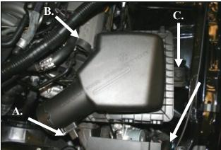
3. A) Slide the red tab, and disconnect the wiring harness from the Mass Air Flow sensor (MAF). Carefully pry the harness anchor from the air box using a screwdriver. B) Separate the resonator tube from the stand off attached to the Air box lid. C) Using a 10mm socket, remove the bolt securing the air box to the inner fender and remove the air box assembly. This bolt will be reused in step 9.
