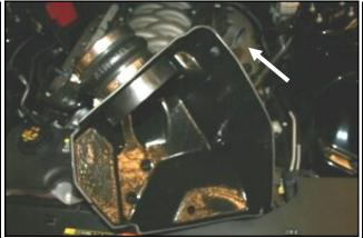
7. Transfer the factory air box mounting grommets. A) 8. Install the hump hose (#4) onto the filter adapter using two #72 hose clamps (#11) as shown. Leave the two hose clamps loose for now. Transfer the resonator stand off from the factory air box into the CAB.
