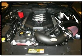
13. Reconnect the Mass Air Flow sensor, which is now 14. Install the Weather Strip (#7) onto the CAB with the located in the lower back side of the intake. Slide the contoured edge going away from the filter. Start at the front of the vehicle and work your way back. Replace the
