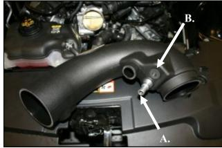
transmission equipped vehicles will also use the 3/8" Fitting (#17) and 3/8" Grommet (#20). Manual transmission vehicles will not need the 3/8" components and will use the Blind Grommet (#21).
