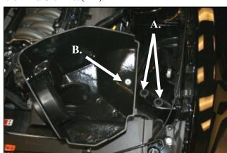
Locate and remove the Two Lower air box mounting grommets, and install them in the inner fender. B) Remove the Upper air box mounting grommet and steel sleeve, and re-install into the Airaid CAB.
