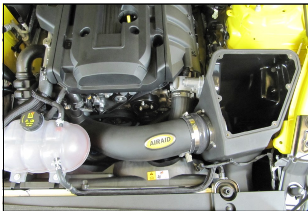
16. Insert the large end of the Intake Tube into the Hump Hose and tighten all 4 Intake Clamps at this time.
