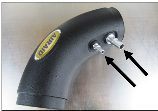
5. Install the Grommets and Aluminum Fittings into the Airaid Intake Tube.
