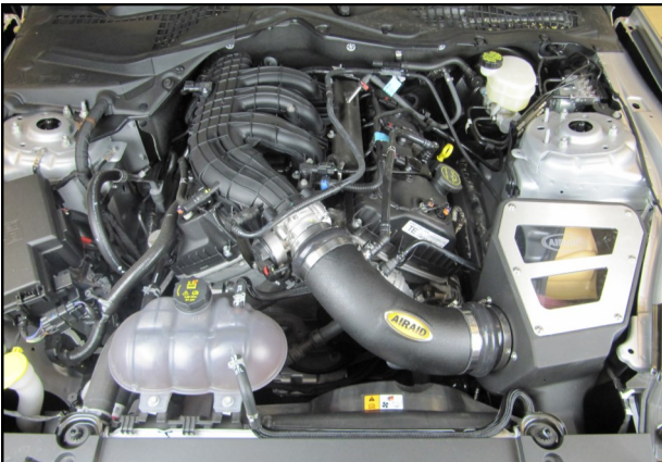
14. Double check your work. Make sure all clamps, hoses, bolts, and screws are tight. Double check the hood clearance. Reconnect the negative battery cable and reinstall the cover.
