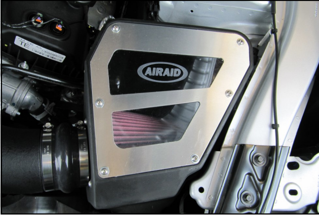
13. Remove the protective film from the Lid and Window before installation. Install the Airbox lid and Window onto the Airbox using 6 sets of 1/4" Button Heads.
