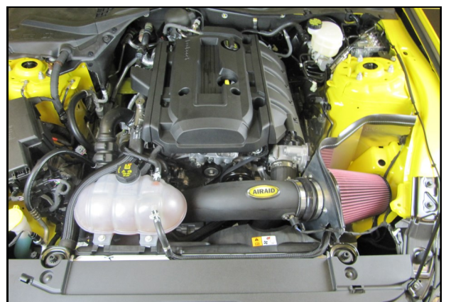
7. Double check your work. Make sure all clamps, hoses, bolts, and screws are tight. Double check the hood clearance. Reconnect the negative battery cable.
