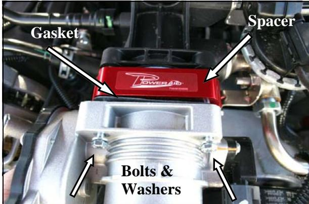
3. Install two bolts (#2), and washers (#3) thru the throttle body, thru the gasket (#4), thru the Poweraid Spacer (#1), and into the intake manifold as shown. **Use caution to retain the factory o-ring gasket on the plastic intake manifold.** Next install the remaining bolts in the bottom holes of the throttle body, and tighten evenly to the manufacturer's specifications. **Do Not Over Tighten The Bolts!**
