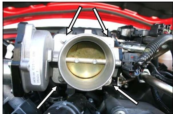
**2. Using a 5/16" socket, remove the 4 bolts that hold the throttle body to the intake manifold.**
