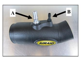
**4.** Install the Grommet and Fittings into the Modular Intake Tube as shown. **A)** All models will require the use of the 5/8" Fitting and the 5/8" Grommet. **B)** Automatic transmission equipped vehicles will also use the Barbed Fitting. Apply the Airaid Decal as shown.
