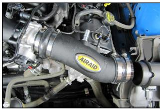
9. Slide the Tube assembly onto the throttle body.
