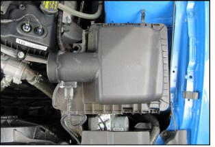
**8.** Unclip the factory air box lid and slide it off of the tabs in front. If you are installing an Airaid Jr. kit, install the Airaid Premium filter at this time. Leave the air box lid unattached for now.
