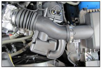
**3.** Loosen the hose clamps on the factory intake tube and remove it.
