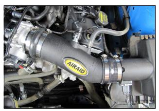
**10.** Slide the air box outlet into the Coupler. Connect the breather lines from step 2 to the Airaid Intake Tube. Rotate the tube if necessary to clear the Hood and valve cover and tighten all Clamps.
