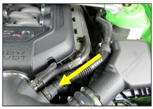
**12. Resonator Delete Install Option:** Airaid has made it possible to eliminate the factory induction resonator if you so desire. The removal of the resonator from the intake has no negative effect on the performance of this kit.
