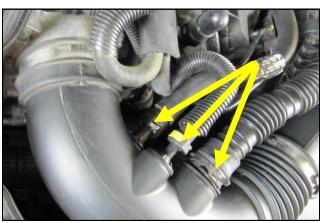
**3.** Compress the spring clamp and disconnect the resonator from the air intake tube. Carefully depress the connector lock tabs, and disconnect the crank case breather line and the brake aspirator line if equipped, (AT models only).
