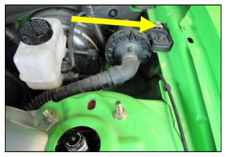
**13.** Remove the entire Resonator tube assembly and all associated stand offs from the intake tube and the vehicle. Remove the 6mm bolt securing the diaphragm housing to the inner fender remove the tubing from the Fire wall.
