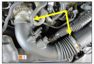
**4.** Loosen the hose clamps on the factory intake tube and remove it. If installing an Airaid Jr. kit, install the Airaid Premium filter into the factory air box at this time.
