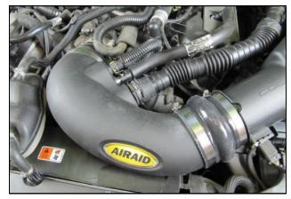
**10.** Connect the breather lines from step 3. to the Airaid intake Tube.
