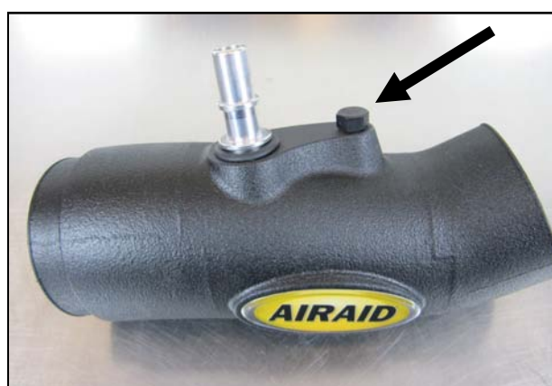
5. Manual transmission vehicles will not need the Barbed Fitting and will use the Threaded Plug.
