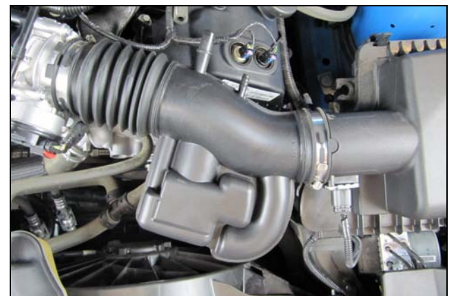
3. Loosen the hose clamps on the factory intake tube and remove it.
