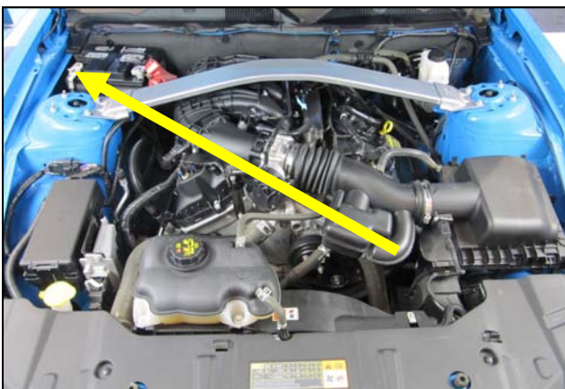
1. Disconnect the negative battery terminal.
