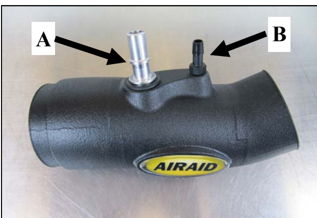
4. Install the Grommet and Fittings into the Modular Intake Tube as shown. A) All models will require the use of the 5/8" Fitting and the 5/8" Grommet. B) Automatic transmission equipped vehicles will also use the Barbed Fitting.
