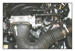
**2.** Loosen the intake tube hose clamp on the throttle body. Slide the red tab on the electrical connector, and disconnect the mass air sensor.
