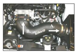
**15.** A.) Install the tube into the hump hose. B.) Now slide the oval coupler onto the throttle body. Tighten the remaining two hose clamps, and re-connect the mass air sensor, from step #2.
