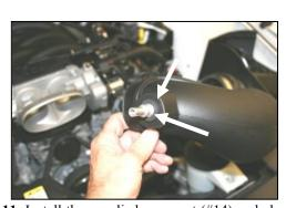
11. Install the supplied grommet (#14) and aluminum fitting (#17) into the Airaid intake tube as shown.
