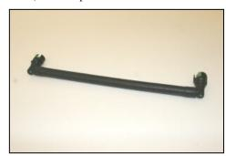
**18.** Install the 3/8"x12" hose (#8) onto the factory breather ends as shown.
