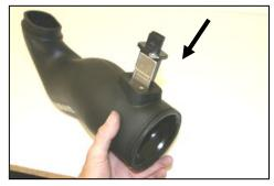
13. Align the two slots in the tubes, and install the factory mass air sensor removed from step #5. Make sure the screw holes line up, then install the two supplied button head screws. (#13). DO NOT USE THE FACTORY SCREWS!!
