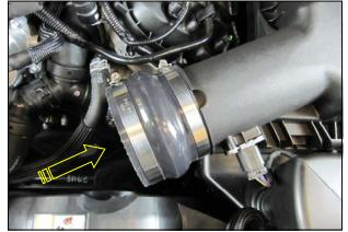
5. Slide the Hump Hose and Clamps onto the airbox outlet as shown. Do not tighten the clamps at this time.
