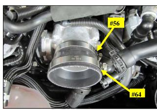
6. Slide the Reducer and Clamps onto the throttle body as
