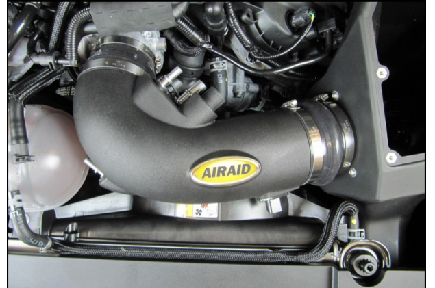
15. Insert the Intake Tube into the Hump Hose and Reducer then tighten all 4 Intake Clamps.
