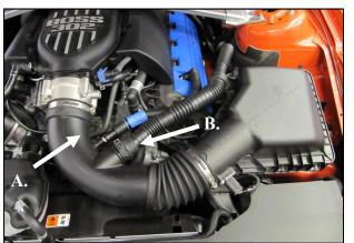
2. A) Loosen the hose clamps on the factory intake tube B) Squeeze the clamp and disconnect the resonator from the air intake tube. C) Carefully depress the hose lock tab and disconnect the crank case breather line. D) Remove the factory intake tube.
