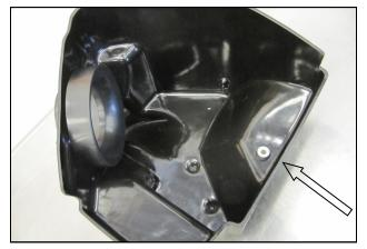
**10.** Remove the factory upper air box mounting grommet and steel sleeve, and re-install into the Airaid **CAB**.
