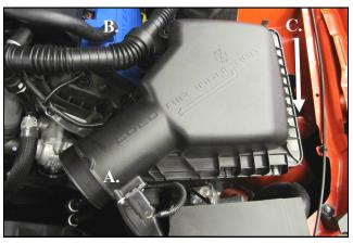
**3. A)** Slide the red tab out of the connector and disconnect the Mass Air Flow sensor. Carefully pry the harness anchor from the air box using a standard screwdriver. **B)** Separate the resonator tube from the stand off attached to the Air box lid. **C)** Using a 10mm socket, remove the bolt securing the air box to the inner fender and remove the air box assembly. This bolt will be reused in step 12.
