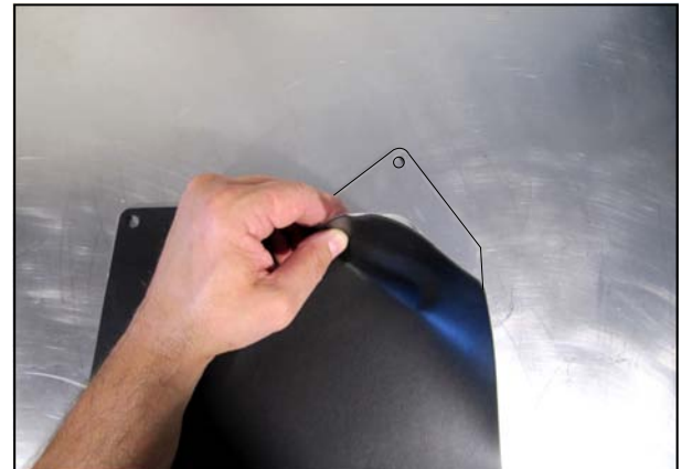
24. Prepare the Airbox Lid for Gasket installation by cleaning the mounting surface using a Prep Solvent or equivalent. Remove the adhesive backing from the Gasket and carefully apply it as shown with the screw holes aligned.
