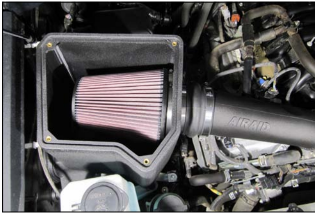
23. Install the Airaid Premium Air filter onto the Filter Adapter inside the airbox.
