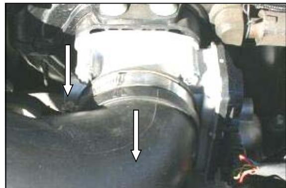
**2.** Using a 10mm socket, loosen the hose clamp on the throttle body end of the intake tube. Slide the intake tube off of the throttle body towards the radiator.
