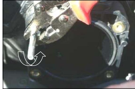
4. Using a stud remover or pair of pliers, carefully remove the factory stud from the intake manifold.
