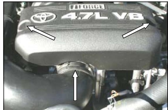
6. Re-install the intake tube and engine beauty cover. **Reconnect the negative battery cable!**
