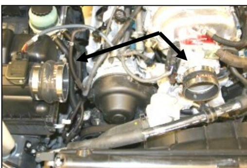
7. Install the hump hose (#3) onto the factory airbox, small end first, with two hose clamps (#6). Next install the reducing coupler (#4), small side first, onto the throttle body with two hose clamps (#7). Leave the clamps loose.
