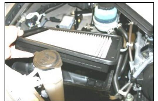
6. Remove the factory air filter, and install the Airaid Premium Filter (#1). Reinstall the factory airbox lid, and latch 4 clips.
