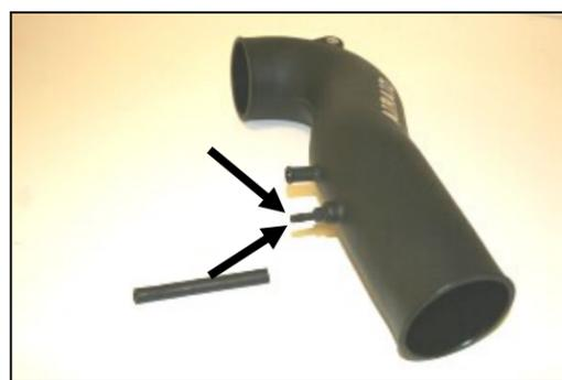
8. Install the 1/4" barb fitting (#10) into the Airaid Modular Intake Tube (#2) as shown. Now slide the 1/4" x 4" hose (#8) onto the barb fitting.
