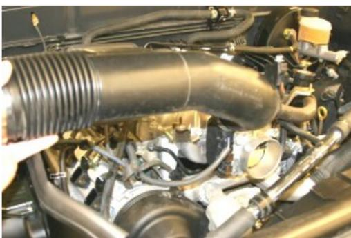
4. Remove the factory intake tube from the vehicle.
