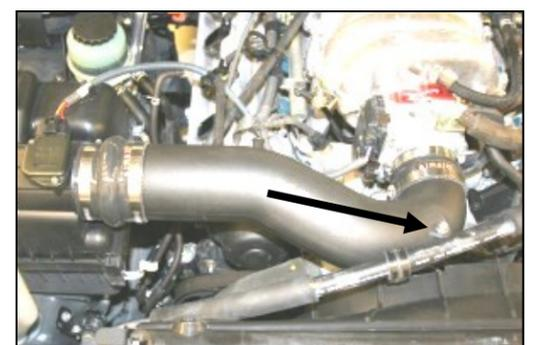
9. Install the MIT into the hump hose first, and then into the reducing coupler. Adjust the MIT snugly against the throttle body, and tighten the 4 hose clamps. Next install the supplied button head bolt (#12) and washer (#11) thru the Adel clamp and into the MIT to hold the air conditioning hose.
