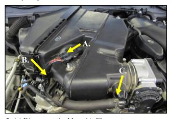
**3. A.)** Disconnect the Mass Air Flow meter. **B.)** Pry the wire harness anchor out of the airbox. C.) Disconnect the crankcase breather line.
