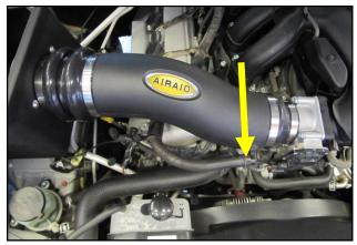
**13.** Connect the factory crank case breather line to the 3/8 Barbed Elbow on the Intake Tube.
