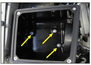
7. Mount the Cold Air Box onto the CAB Mounts using the three 8mm Bolts (#14) and 5/16 Flat Washers
