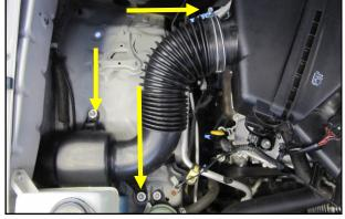
2. Loosen the clamp on the factory intake tube and remove the two 8mm bolts securing the other end on the inner fender. Slide the intake tube out from the inner lender hole and set it aside.
