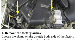
airbox and remove the two 6mm bolts securing it to the motor. Remove the entire airbox assembly from the ve-
