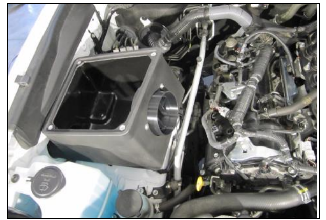
12. Position the Airaid Airbox assembly into the engine compartment as shown.
