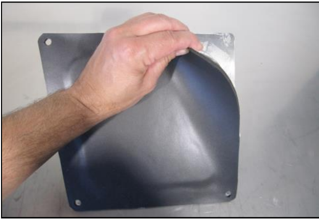
10. Prepare the Airbox Lid for Gasket installation by cleaning the mounting surface using a Prep Solvent or equivalent. Remove the adhesive backing from the Gasket and carefully apply it as shown with the screw holes aligned.
