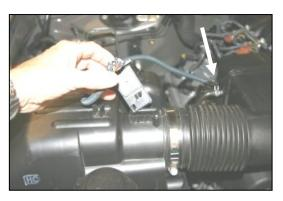
SECURES MAF SENSOR CONNECTOR CABLE (21)
