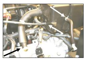
**12.** Disconnect breather hose from valve cover. Disconnect 1/8" vacuum line, and 1/4" vacuum line from the back of the factory intake tube.
