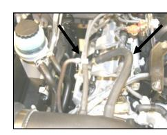
**18.** Install the vacuum tee (#13) into the 1/4"x4" hose (#14), and reconnect the factory 1/4" and 1/8" vacuum lines to the tee as shown. Install the 1/2"x13" breather hose (#8) onto the valve cover and to the MIT as shown.
