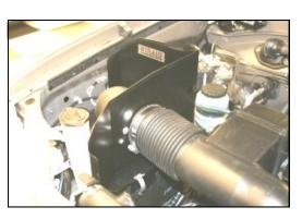
7. Slip MAF adapter into factory intake tube while installing CAD onto top of factory airbox. Adjust for fit, and latch 3 factory clips on factory airbox. Tighten the hose clamp on the intake tube. Replace the fan shroud bolt that was removed in step #5.
