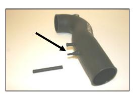
**16.** Install the barbed fitting (#11) into the MIT as shown, and then slide the 1/4"x4' hose (#13) over the fitting.
