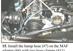
**15.** Install the hump hose (#7) on the MAF adapter (#4) with two hose clamps (#11). Install the reducer (#6), small end first, onto the throttle body with two hose clamps (#10). Leave the clamps loose for now.
