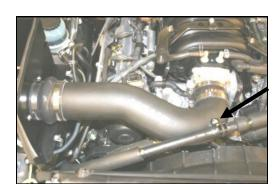
17. Install the MIT (#5) into the hump hose (#7), and then into the reducer (#6). Adjust the MIT snugly against the throttle body, and tighten all 4 hose clamps. Install the supplied button head bolt (#18), and washer (#19), thru the Adel clamp and into the MIT to hold the air conditioning hose.
