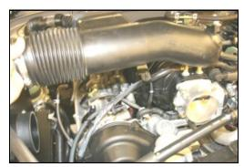
14. Remove the factory intake tube.
