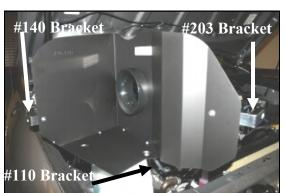
7. Assemble the Cool Air Dam panels (#3 & #4) as shown using four 6-32 screws (#9), washers (#10), and keps nuts (#11). Install the filter adapter (#5) using three 1/4" button head bolts (#13) and washers (#14). Install the 3 brackets (#24), (#25), and (#26) as shown using three 1/4" bolts (#13), washers (#14), and nuts (#15). Just snug the bolts for now, they will be adjusted later.
