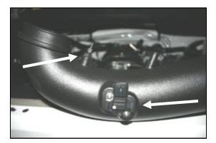
10. Install the 1/8" barbed fitting (#20) into the Airaid intake tube (#2) as shown. Next install the MAF sensor removed in step #9, into the Airaid intake tube and secure it with two 8/32" x 3/8" (#12) button head screws. Do Not Use The Factory Screws!
