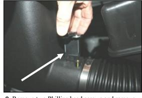
**9.** Remove two Phillips head screws and remove the **MAF** sensor from the factory intake tube. It will be reinstalled in step #10.
