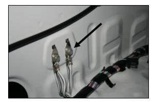
**6.** Using a 10mm socket, remove the rear ground anchor bolt on the passenger side inner fenderwell. Save the bolt, it will be reused in step #8.
