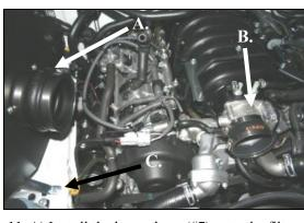
11. A) Install the hump hose (#7) onto the filter adapter using two #72 hose clamps (#19). B) Install the smaller end of the reducer coupler (#6) onto the throttle body using one #52 hose clamp (#17). Next install the #56 hose clamp (#18) over the coupler and leave it loose. C) Now align the #110 bracket (#24) over the captured nut in the fender well and install one 6mm bolt (#16) and washer (#14). Leave loose until final adjustment.
