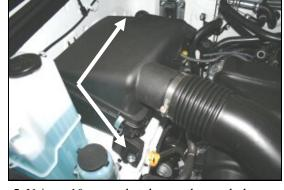
**5.** Using a 10mm socket, loosen the two bolts that anchor the factory airbox to the inner fenderwell. One is on the front of the airbox, and the other is on the rear. Pull the factory intake tube away from the throttle body and remove the complete factory intake assembly from the vehicle.
