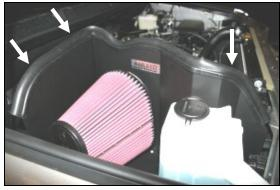
14. Install the Airaid Premium Filter (#1) onto the filter adapter and tighten the clamp. Next install the weather strip (#8) on top of the CAD as shown. For an easier install, start at the fender side of the CAD and work your way towards the radiator. Reinstall the factory beauty cover.
